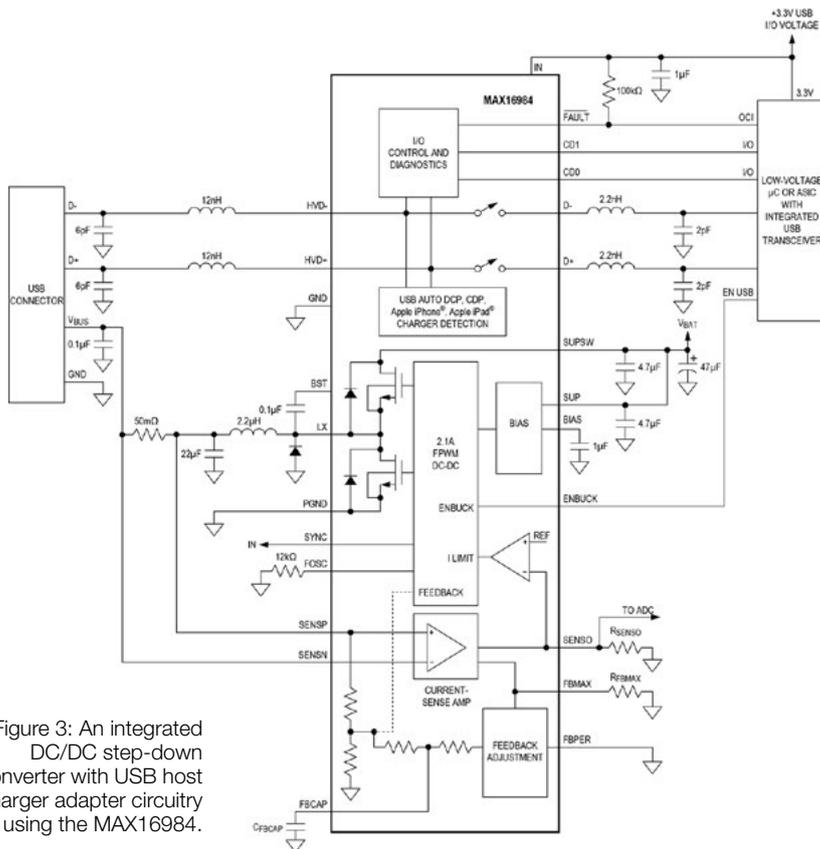
Figure 3: An integrated DC/DC step-down converter with USB host charger adapter circuitry using the MAX16984.
