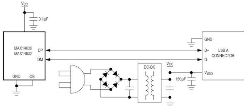
devices can be charged using an adapter emulator to communicate current limits.
