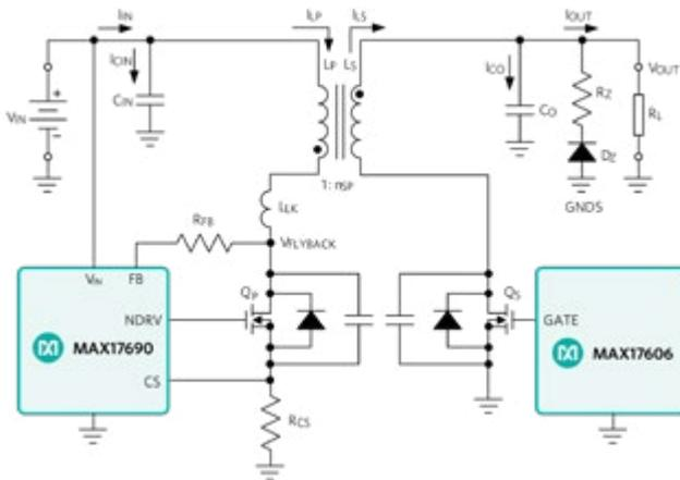
Figure 2: Simplified No-Opto Flyback Schematic with Synchronous Rectification
