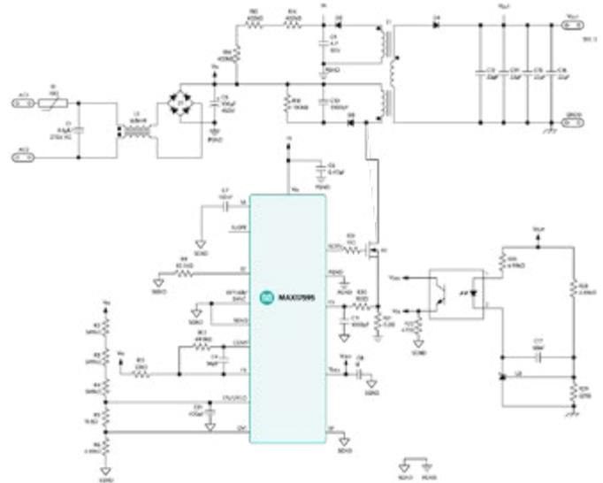
Figure 4: AC-DC Power Supply
