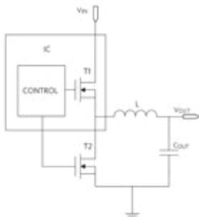
Figure 3: Simplified Synchronous Buck Architecture
