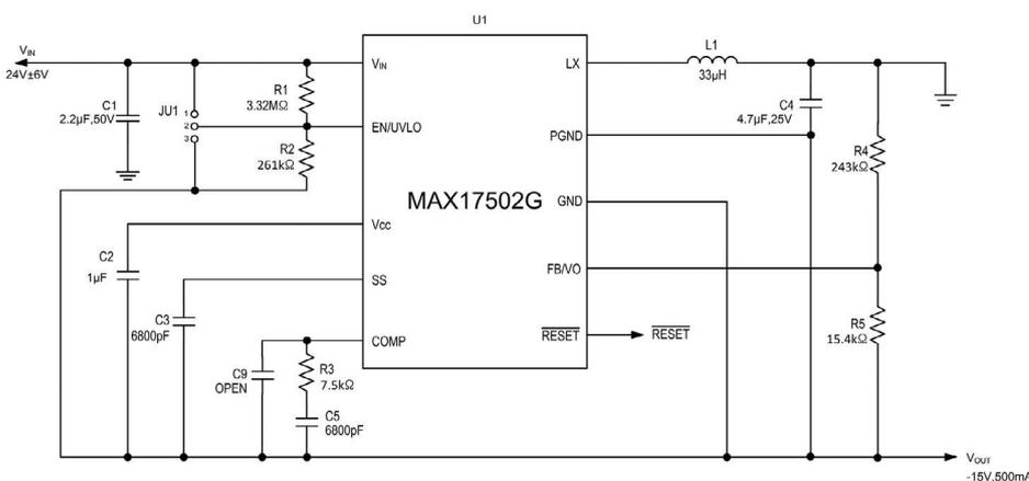
Figure 1: Schematic for a +18V to +30V/-15V positive-to-negative output voltage converter using the MAX17502.
