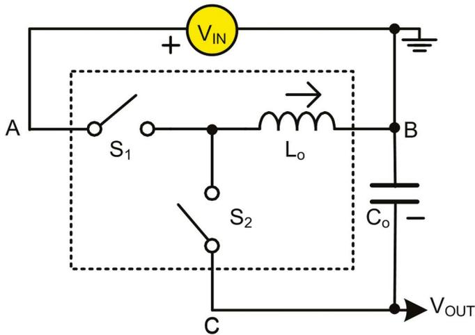
Figure 3: Simplified schematic of the synchronous inverting buck-boost converter.
