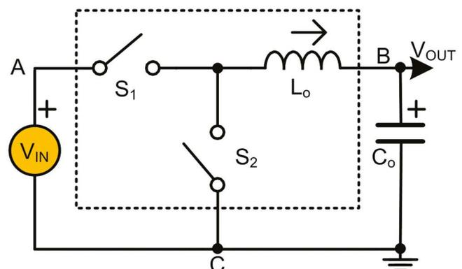
Figure 2: Simplified schematic of the synchronous step-down converter.
