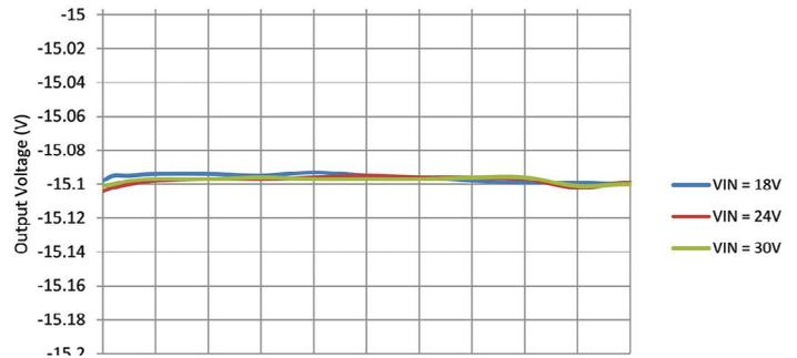
Figure 5: Load and line regulation of output voltage
