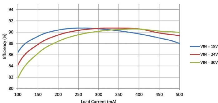
Figure 4: Efficiency vs. load current.
