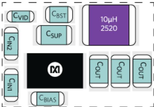
Figure 6: Integrated Smart Hub Power Solution with MAX77756 (33mm<sup>2</sup>)
