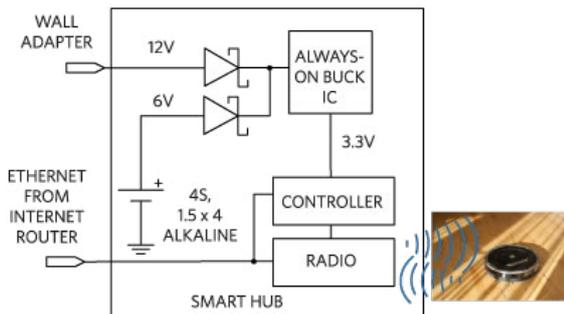
Figure 2: Typical Smart Hub System
