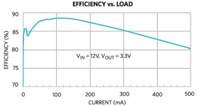
Figure 7: MAX77756 Efficiency Curve
