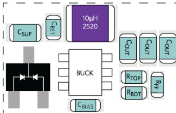
Figure 3: Typical Smart Hub Power Section Footprint (46mm<sup>2</sup>)
